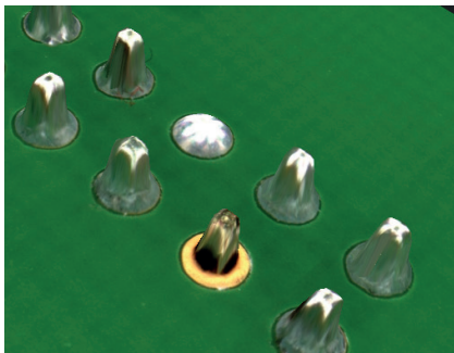
Insufficient wetting (front) and missing pin (back)
