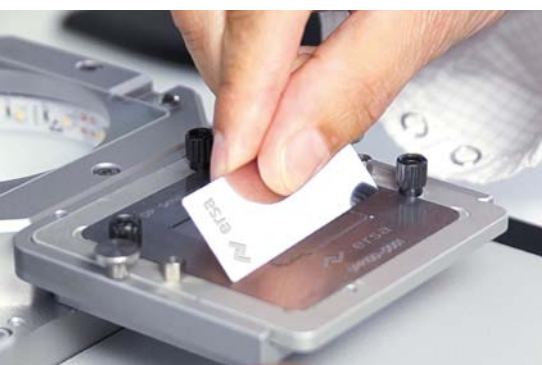
Flux deposition in the dip stencil
