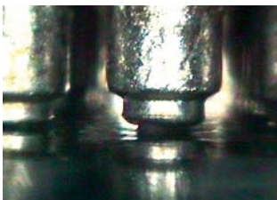
CCGA: insufficient solder
