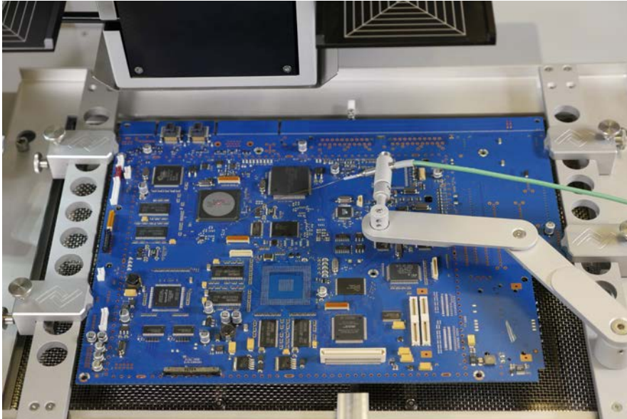
Processing an assembly in the HR 550
