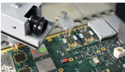
Live process monitoring on the HR 600 XL
