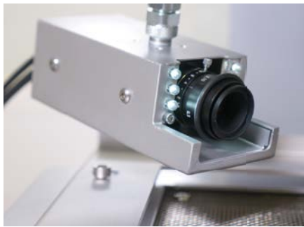
Reflow Process Camera (RPC) on the HR 550
