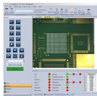
Superimposing of component and target position
