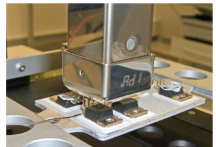
TO220 on aluminium carrier with hybrid rework system
