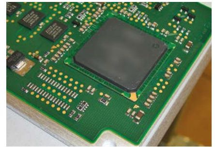
PBGA on aluminium carrier
