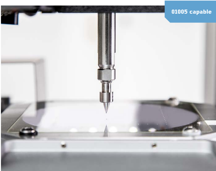
Automatic pick-up of a 01005 chip
