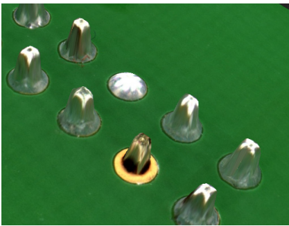
Insufficient wetting (front) and missing pin (back)
