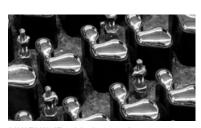
${\it MULTIWAVE soldering\ nozzles}$
