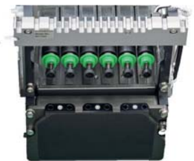
Laser sensor integrated into placement head
