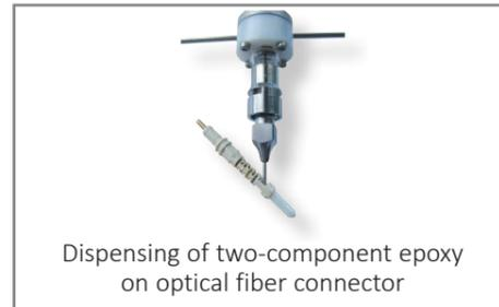
Dispensing of two-component epoxy on optical fiber connector
