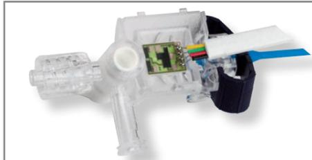
Laser soldering of wires on a ceramic substrate of a medical pressure sensor
