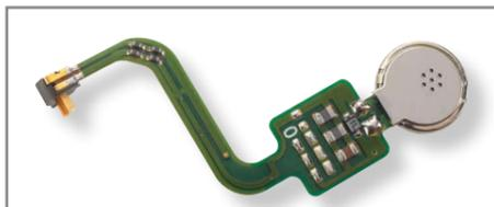
Iron soldering of a microphone and connector for mobile telephone
