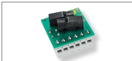
Iron soldering of terminals on a printed circuit
