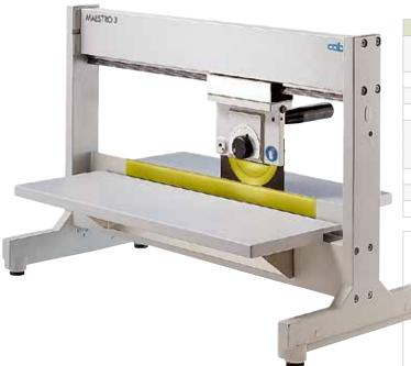
**Technical Data** Separation type Component side circular blade Solder side linear blade by hand Operation Separation length max. 450 mm Material FR4, Aluminum Temperature/ Operation + 5 - 40°C / 10 - 85% Humidity Storage +0-60°C/20-80% Transport - 25 - 60°C / 20 - 80% not condensing Weight 455 x 700 x 350 mm Dimensions H x D x W CE, FCC class A Approvals
