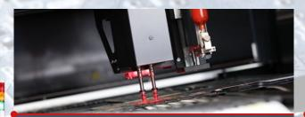
Configurable heads with 1-4 placement-axis. 2,5D and 3D dispensing and jetting, High resolution digital vision system with auto component teach-in and irregular ball recognition.
