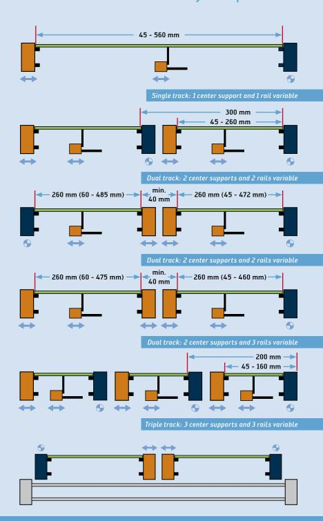
As an alternative to the center supports, the conveyors could also be equipped with a low mass tubular support safety conveyor running below the conveyor rails (example shows safety conveyor below dual track conveyor).
