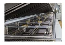
In modern reflow systems, the efficiency of the heat transfer exerts an important influence on all matters related to quality, productivity and operational cost, which, together, directly impact on the profitability of the process. It is just for this reason that in the HOTFLOW 4 model line, special attention was being paid to further optimize the heat transfer rate.
