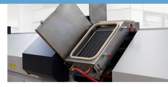
Cleanliness of the process zone is of supreme importance in the reflow process, since it determines the uptime of the system and ensures a stable and reproducible process. Contaminations in the process gas atmosphere stem from various sources. The two most important are the solder pastes and the base material of the printed circuit board.
