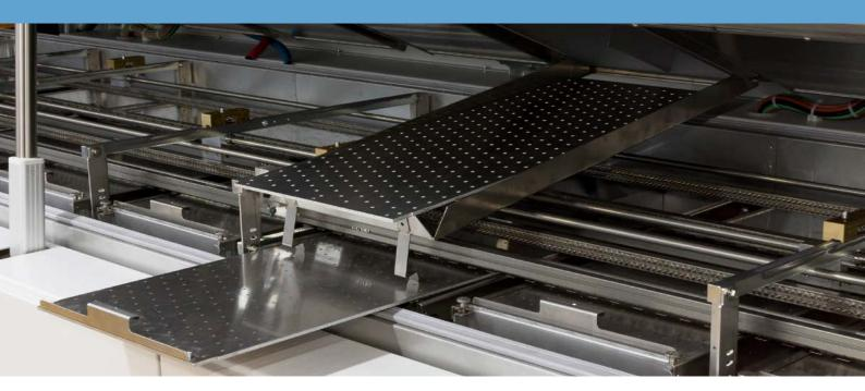
Ease of maintenance and serviceability, as well as the total time required to perform the necessary maintenance, play a major role when looking at the performance capability of a modern reflow soldering system. But, for a user, performing maintenance means that during this time the system is not in productive operation.
