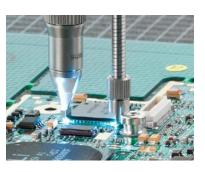
ERSASCOPE 2: exchangeable optics for CSPs
