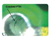
Plated thru-hole: cracked wall
