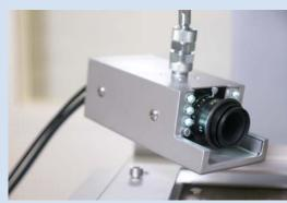
Reflow process camera on the HR 550
