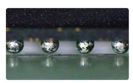
Real-time rework process visualization of BGA during reflow
