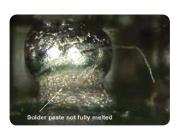
PBGA – scaling: insufficient heat
