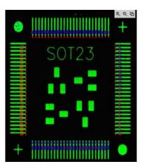
Computer-supported alignment of a QFP
