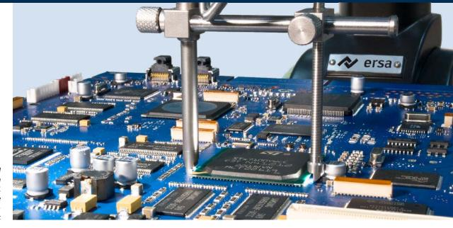
Integrated front and back lighting allows for optimal illumination of the hidden joints underneath the component
