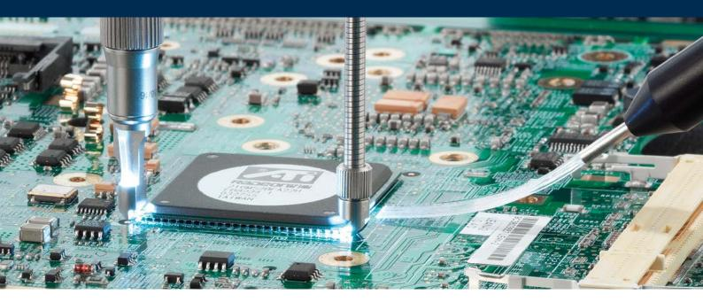
Optimal component illumination is essential for a quality inspection process
