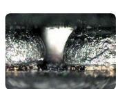
PBGA – scaling: insufficient heat
