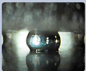
ERSASCOPE 2 image of Flip-Chip (gap  $\sim$  30  $\mu$ m)
