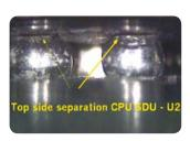
Top-side delamination of BGA
