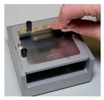
Flux deposition in the dip stencil
