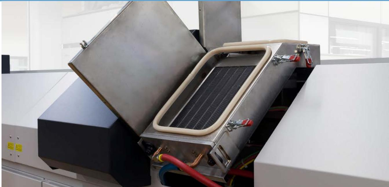
Cleanliness of the process zone is of supreme importance in the reflow process, since it determines the uptime of the system and ensures a stable and reproducible process. Contaminations in the process gas atmosphere stem from various sources. The two most important are the solder pastes and the base material of the printed circuit board.
