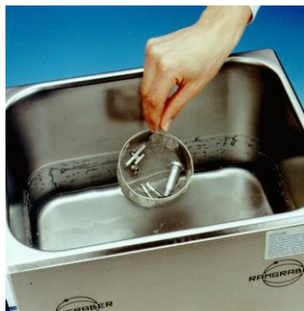
Cleaning of dispensing needles with ZESTRON® ES 200 in an ultrasonic tank
