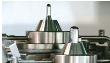
*Dual solder pots with soldering nozzels in different shapes*
