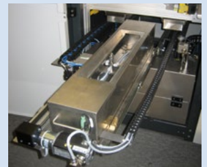
Maintenance-friendly spray fluxer designed to meet highest demands in lead-free soldering
