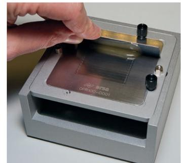
Flux application in a dip stencil
