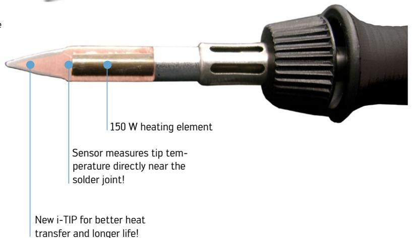
The i-TOOL recovers so fast that all solder joints can be made with nearly the same temperature. The sensor measures the actual tip temperature very close to the tip extremity. The Process Window Alarm enables a repeatable soldering quality for the operator.
