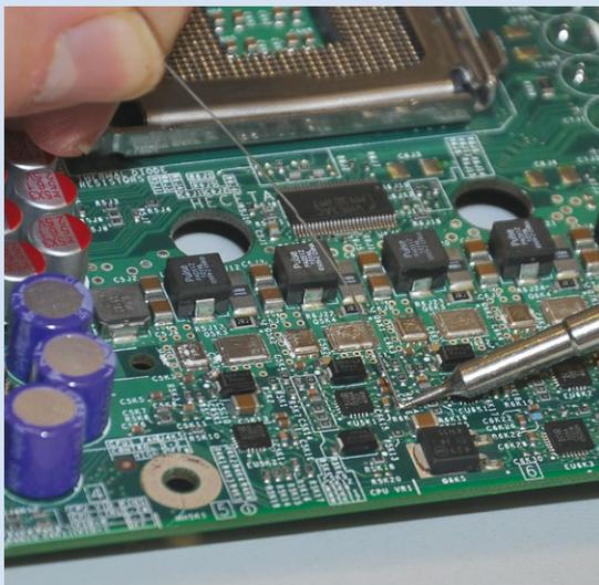
The soldering tip is the "heart" of the soldering iron and responsible for the heat transfer from the heating element via solder to the solder joint.
