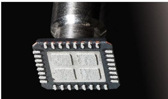
MLF 32 with solder paste printed on the bottom
