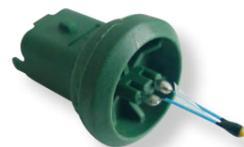
Induction soldering of a temperature sensor
