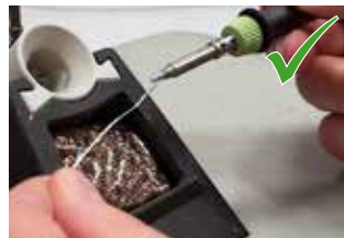
Add new solder after cleaning
