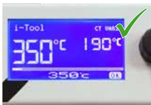
340 – 360 °C for lead-free solder
