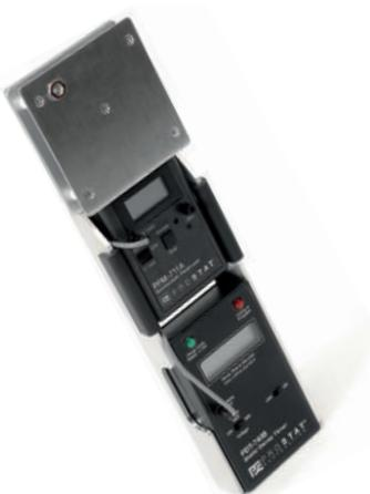
Allowing measurements of electrostatic field - discharge time. Ideal for calibrating and qualifying ionisers:
