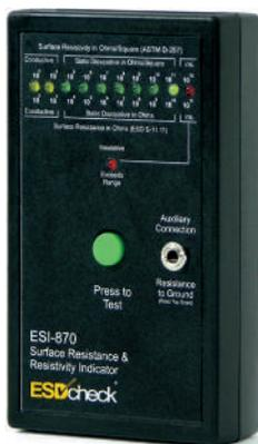
Portable tester that measures surface resistivity and resistance to ground of surfaces in accordance with ASTM D-257 norm by using parallel electrodes.
