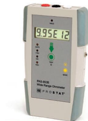
Large spectrum portable  $\Omega$  meter: from  $0.01 \Omega$  to  $9,99 \times 10^{12} \Omega$  (+/- 5%).
