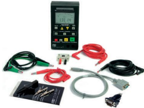
Accurate Wide Range Resistance Measurements:  $0.1 \Omega$  to  $2.0 \times 10^{14} \Omega$ . Measures constant voltage, wide range ohmmeter with data logging, calculating and computer communication capabilities.
