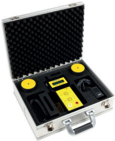
Tera-Ohm meter that can measure from  $10^4\Omega$  to  $10^{12}\Omega$ . Measures resistance, temperature and humidity at the same time.
