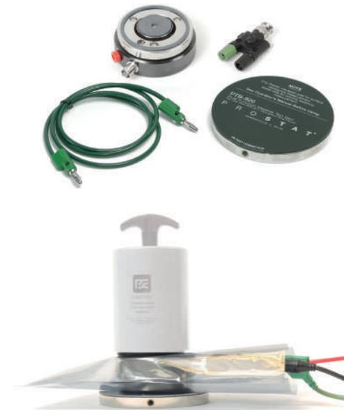
Allows to measure surface resistance and volume resistance of flat materials in accordance to IEC 61340-2-3.
