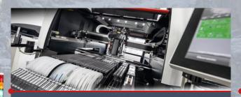
Configurable heads with 1-4 placement-axis. 2,5D and 3D dispensing and jetting, High resolution digital Cognex vision system with auto component teach-in and irregular ball recognition.
