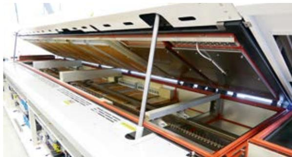
Reflow ovens with nitrogen connection are equipped with a water cooling system to ensure effective cooling and flux separation.
