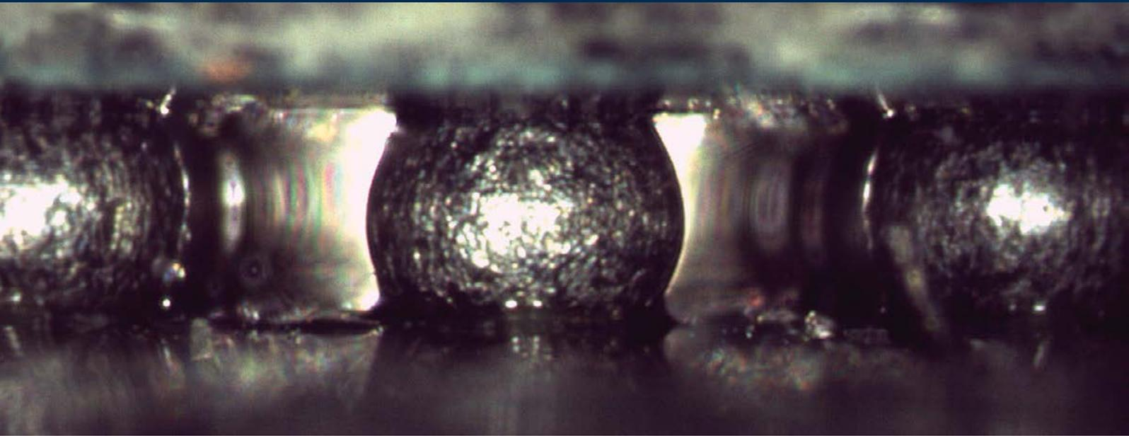
Hidden solder joint inspection is one of the most important areas in a quality assurance program. The images shown on these pages underscore the flexibility of the ERSASCOPE inspection systems.
