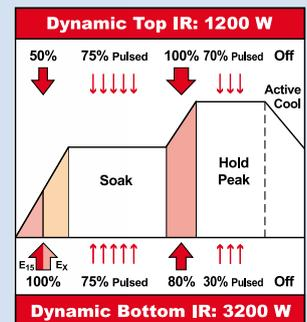
The IR 650 selective reflow module uses DynamicIR heating technology for fully automatic dynamic control of the top (1,200 W / 60 mm x 120 mm) and bottom (3,200 W / 350 mm x 450 mm) IR heaters. The total available power (4,400 W) to the selective reflow system is spread across 4 separately controllable heating zones on the top and 5 zones on the bottom. Depending on board size, the thermal mass of the substrate and
