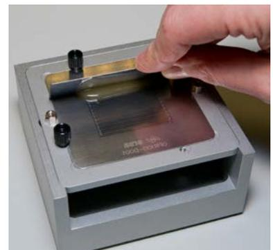
*Flux deposition in the dip stencil*
