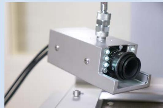
Reflow process camera on the HR 550
