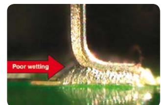
*PQFP: missing interior heel fillet*
