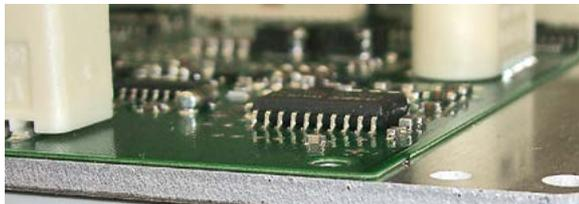
*SOIC and plastic SMT on aluminium carrier*
