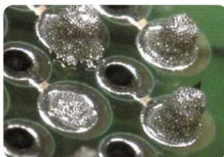
BGA – paste print: insufficient solder
