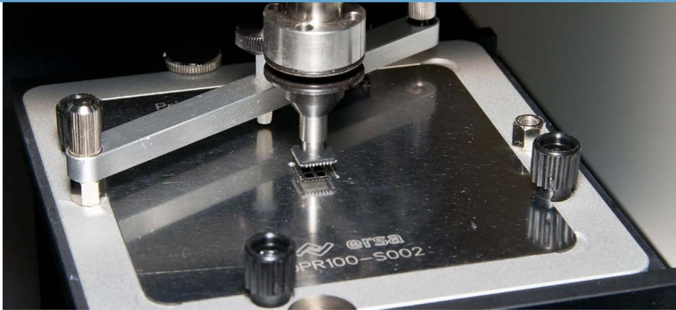
The Ersa Dip&Print Station enables the user of an Ersa rework system to easily, reliably and reproducibly perform the preparatory work on the component (application of solder paste or flux).
