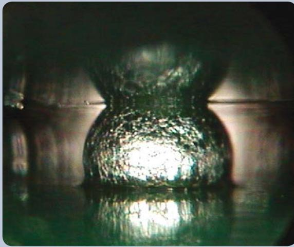
ERSASCOPE 1 image of BGA (gap ~ 300 μm)
