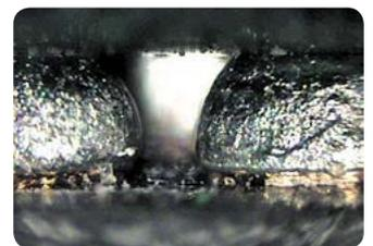
PBGA – scaling: insufficient heat
