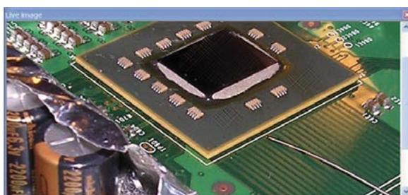
Rework process visualization with live image window
