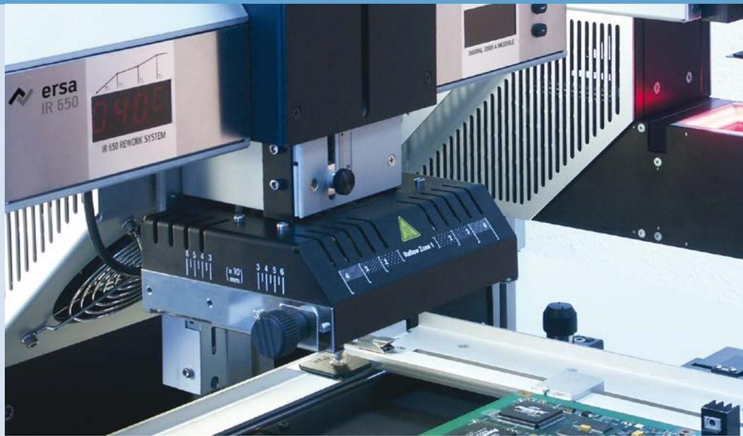
The IR/PL 650 provides a very high heating power (4,400 W) for large and complex PCBs. Offering a high degree of automation, the IR/PL 650 requires only little user intervention. This guarantees stable and repeatable rework processes for all applications.
