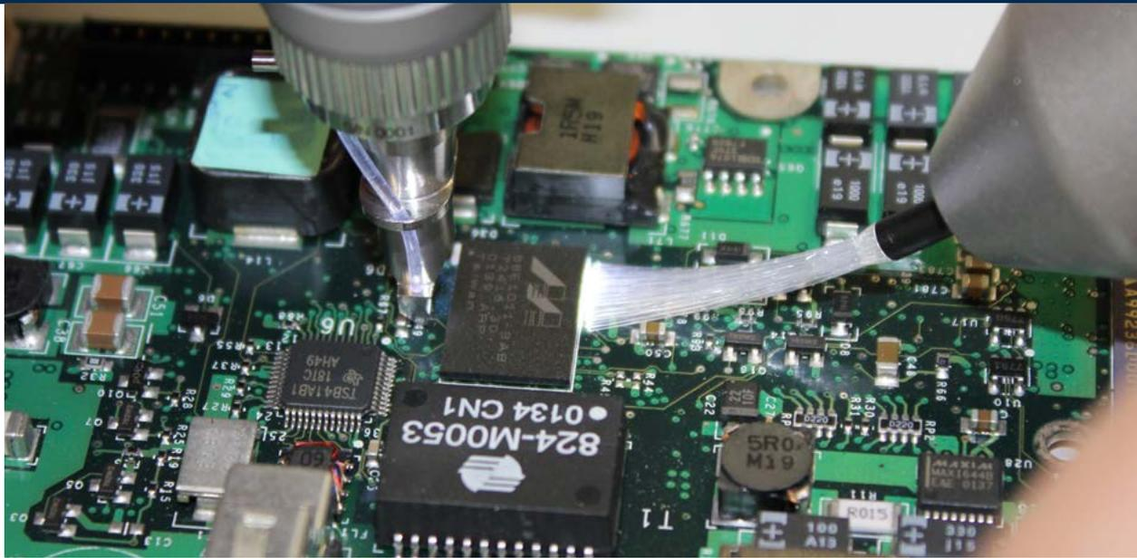
Long-life and very bright, controllable LED lights are integrated in both optical heads and provide optimal illumination of the solder joints. In BGA inspection an additional LED light brush is essential for backlight illumination or to light up very hidden and hard-to-reach areas. Thus soldering errors can be detected quickly and easily with the Erska MOBILE
