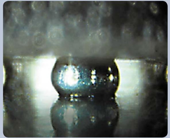
ERSASCOPE 2 image of Flip-Chip (gap ~ 30 μm)
