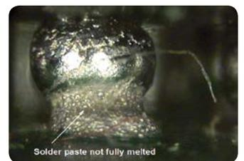
PBGA – scaling: insufficient heat
