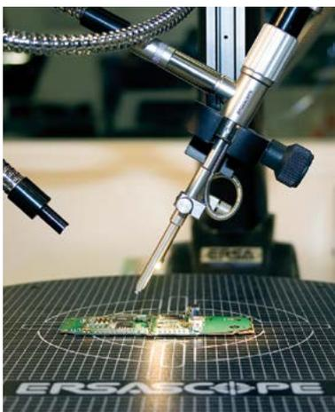
*Integrated front and back lighting allows for optimal illumination of the hidden joints underneath the component*
