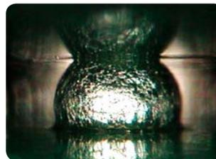
*PBGA – scaling: insufficient heat*
